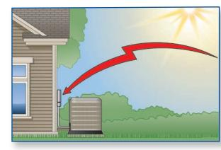
When demand for electricity peaks, we will send a wireless signal that "cycles" the compressors of participants' central air conditioning units and heat pumps. Typically these conservation periods amount to less than 1% of the year.
